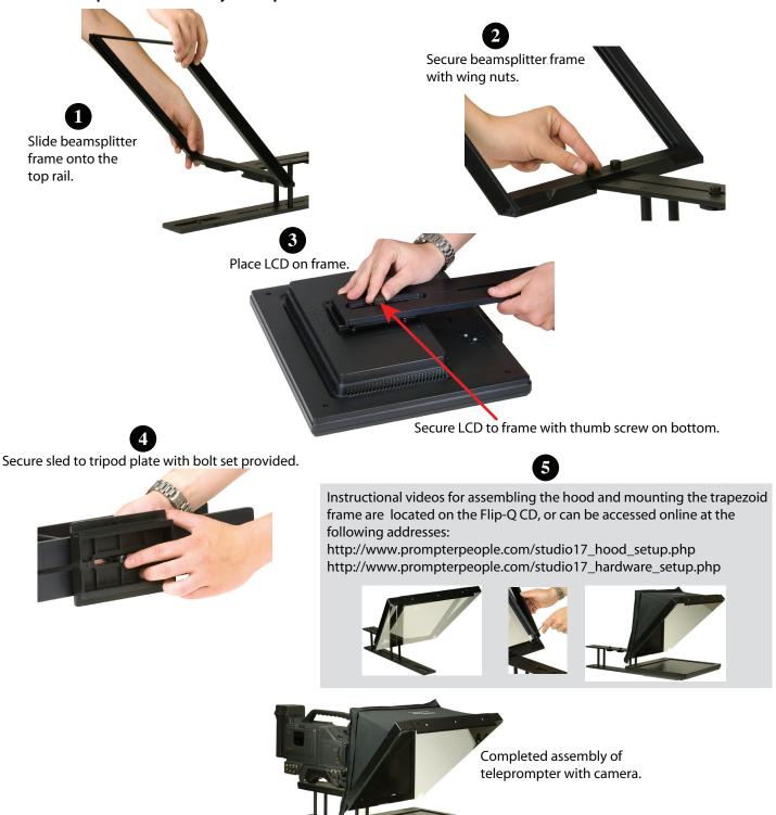
To balance the teleprompter, place a pen under the unit with the camera and all parts attached. Move back and forth to find the balance point. Attach your tripod quick release plate at this point.
