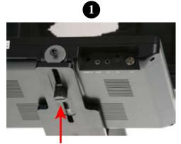
Attach the monitor to the teleprompter sled. Adjust the monitor back and forth until centered.
