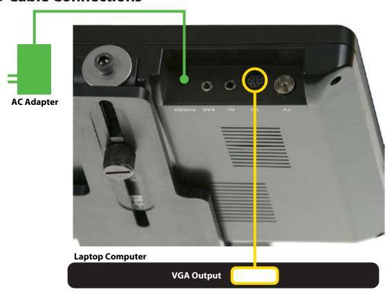
The LCD display comes with a breakout cable to connect power, video and audio.
