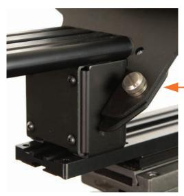
When mirror assembly is firmly seated tighten the two metal knobs on the top side to secure the mirror assembly in place
