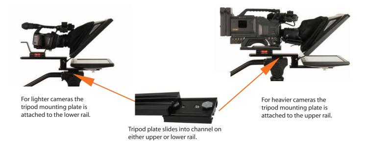
Loosen thumbscrews and lift up retaining plate on back of upper rail to slide on tripod mounting plate.
