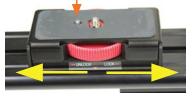
Turn the camera knob to secure camera. Loosen slightly to adjust camera position. When camera is in position turn knob to lock into place. Do not over tighten.
