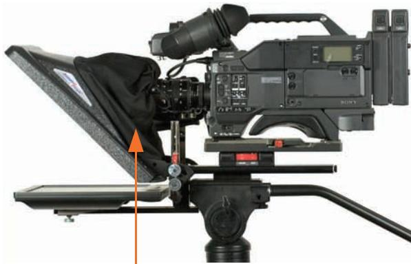
Once camera is positioned place lens shade around lens.
